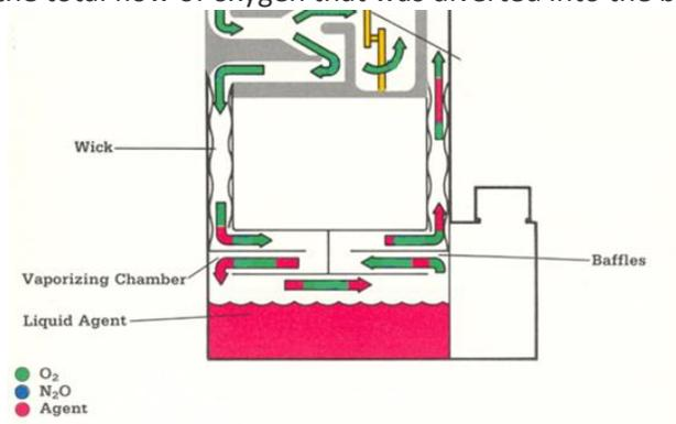
The dial at the top of the vaporizer – the one we use to set our desired percentage of anesthetic gas – actually diverts a percentage of the oxygen flow downward, through the wick and into the sump holding
