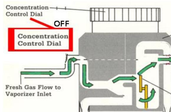
I've stripped away everything but the oxygen flow in this top-half view. I have highlighted the "Concentration Control Dial" label and showed what turning the setting to OFF will do to the oxygen flow. Notice the oxygen just flows straight through the vaporizer with no oxygen diverted into the lower half of the vaporizer.
