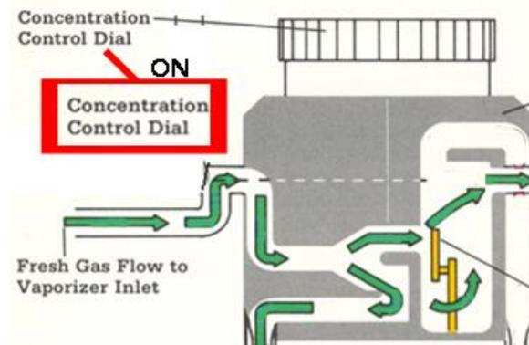
In this view, everything is the same except the highlighted "Concentration Control Dial" is turned ON. Notice a percentage of the flow is diverted into the lower half of the vaporizer, while the majority of the flow still passes directly through and out of the vaporizer. Now let's slide the image a little lower and follow the percentage of the total flow of oxygen that was diverted into the bottom of the vaporizer.
